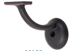
30155 Wall to tip projection: 3-3/4" Wall to center line: 3-3/8" Base diameter: 2-1/8"
